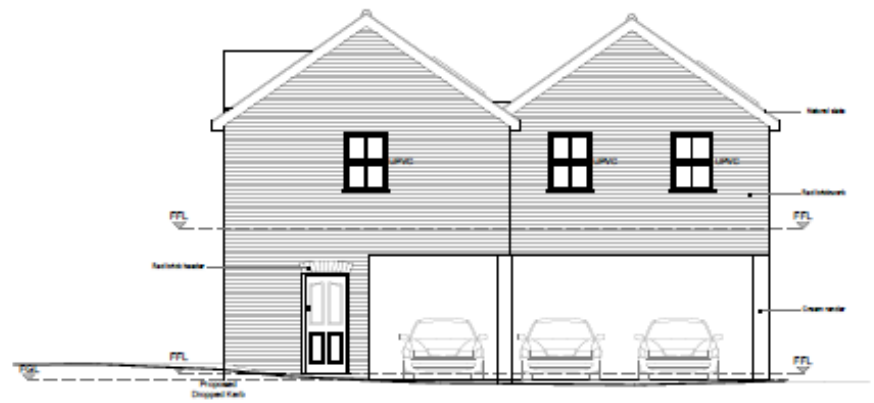
PROPOSED ONE-BED FLATS AT THE REAR - SIDE ELEVATION K-K (SOUTH-WEST) - Scale 1:100 @ A3
