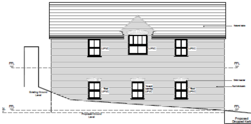
PROPOSED ONE-BED FLATS AT THE REAR - FRONT ELEVATION B-B (NORTH-WEST) - Scale 1:100 @ A3
